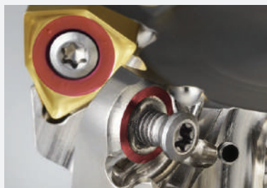
The conical shim surface and the M5 screw for WWX400, and the M3 screw for WWX200 provide a high damping force.
