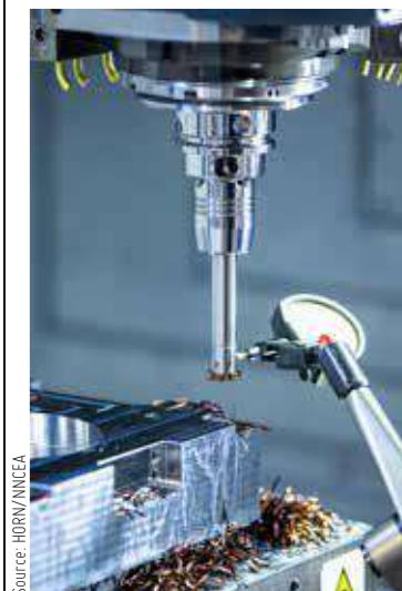
The Tendo Zero clamping system offers precise adjustment of the concentricity.
