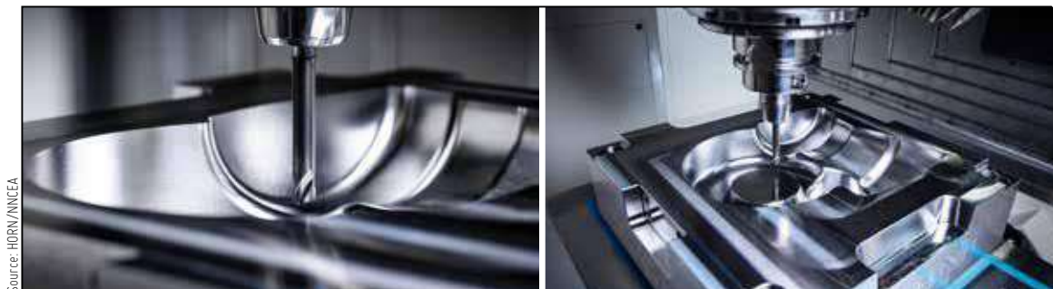
The ball milling cutters of the Horn DS system enable a high achievable surface quality due to their high precision.
