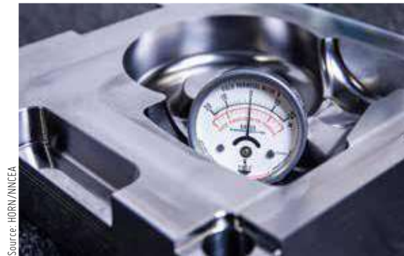
The component itself is not magnetic after clamping.
