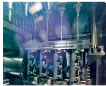
Quadruple machining of fuel supply distributor parts with deep hole drills. The clamping fixtures that rotate in opposite directions to minimize the deviation of the drill are what makes the solution exceptional.
