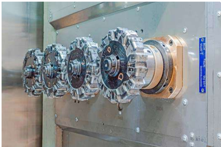
Quadruple application of disc milling cutters on control arms. The solid cutting surfaces provide an indication of the high drive power required.
