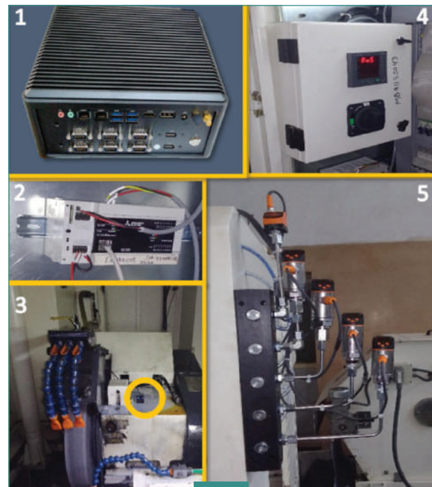
IIoT Hardware integrated on a machine (1 - Edge Device for Data Acquisition, Data Pre-processing, and Cloud Connectivity, 2 - PLC for Data collection from Hardware, 3 - Vibration Sensors for condition monitoring of Wheel Head and Work Head, 4 - Energy Meter for Monitoring Energy Consumption, 5 - Hydraulic Pressure, Pneumatic Pressure, and other IO-Link Sensors for Process and Health Monitoring)
