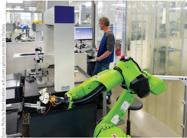
John Loscheider, CMM Programmer, Ultra Machining Company, oversees an automated CMM and multi-axis robot. The inspection data from this CMM is uploaded in real time to the shop floor, allowing machine operators to see whether the parts remain within tolerance requirements.
