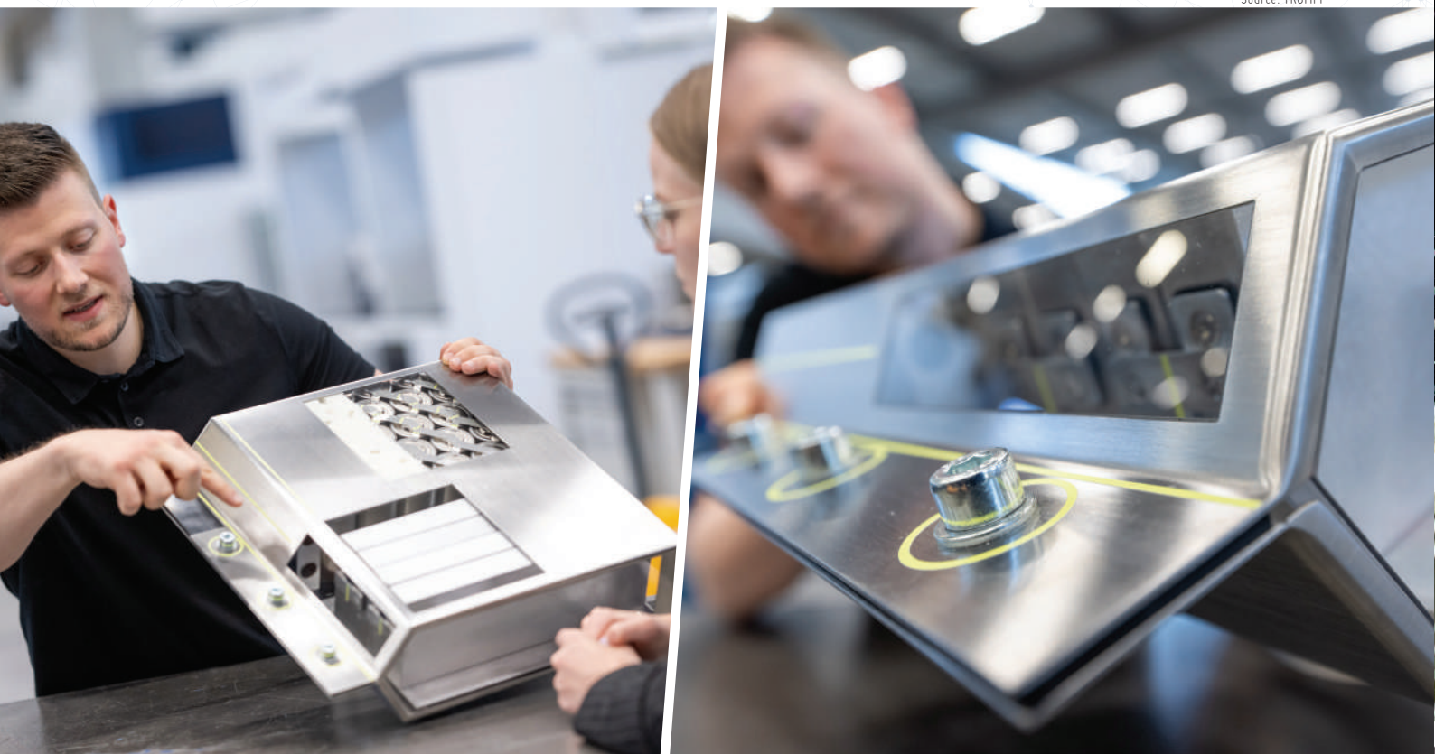
A TRUMPF employee explains where the battery will be cut open by the laser. A TRUMPF employee cutting open used/faulty batteries using laser technology.
