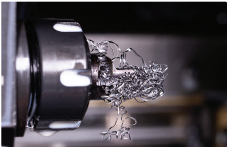
Before switching to the new tool generation, RICH Praezision GmbH often had problems with tangled swarf.
