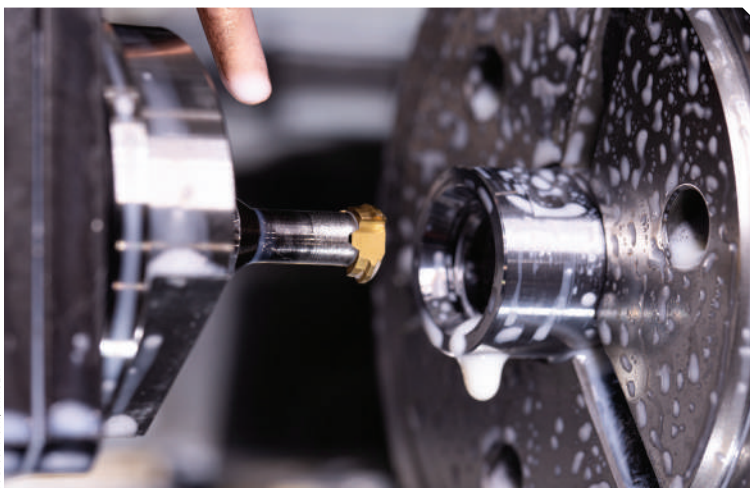
A type 306 insert is used for milling the precision thread.
