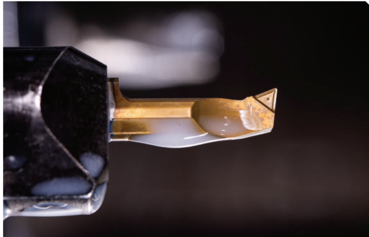
For internal grooving, RICH Praezision GmbH relies on solutions from the Supermini tool family.
