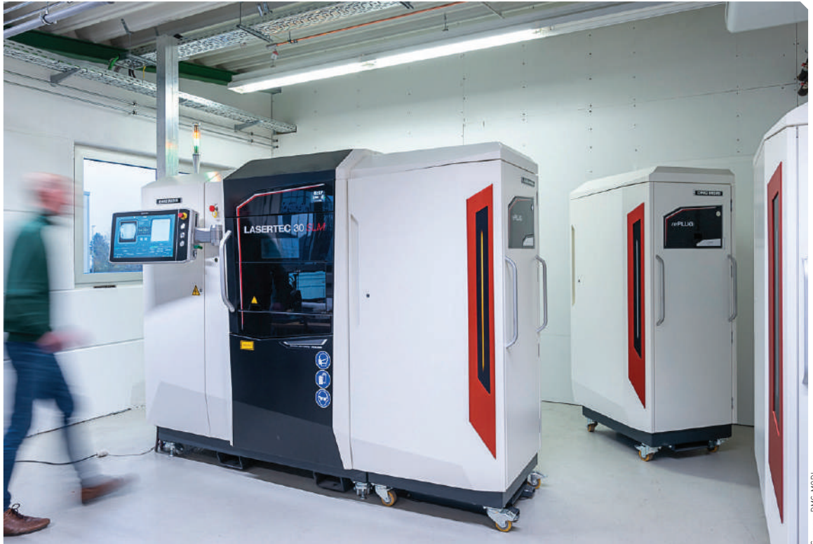
Powder change <2h – The rePLUG powder modules ensure safe powder handling.
