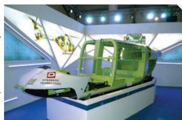
Bell 407 Helicopter Cabin Assembly
