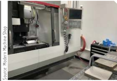
Fig 5: Another capability needed for laser powder bed fusion: milling to resurface build plates.
