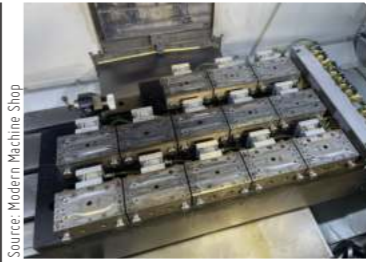
Fig 9: Effective AM for production often will rely on workholding able to batch many parts for quick finish machining. Metal injection molders are already accomplished at this. This photo was taken at Smith Metal Products, a metal injection molder expanding into metal additive manufacturing via binder jetting.
