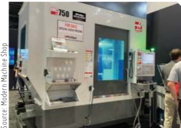
Fig 13: Hybrid machine tools combine additive manufacturing with machining. This example was seen at the most recent International Manufacturing Technology Show. Phillips Corp. adds metal-deposition 3D printing heads to existing machining centers to convert them to hybrid machines.
