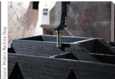
Fig 11: On this large-scale polymer composite form made through additive manufacturing, machining accounts for more of the production time than 3D printing. The part is a nearly complete 3D printed housing for a flight simulator. Making this housing in just a few big 3D printed pieces contributed to an assembly consolidation that reduced the simulator's part count by thousands.
