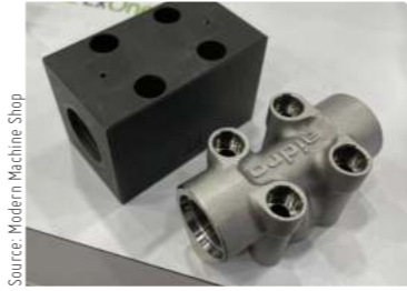
Fig 8: Manifold maker Aidro increasingly makes its components through additive manufacturing rather than by drilling intersecting holes into solid blocks. The company 3D prints manifold parts using both LPBF and binder jetting. (Aidro is part of AM technology provider Desktop Metal).
