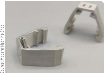
Fig 12: Energy sector spare part maker Sparox 3D used low-cost metal AM via fused filament fabrication to manufacture these solar panel clips as an alternative to machining.
