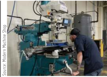
Fig 10: This is actually a picture of additive manufacturing. A simple milling step is vital to AM via laser powder bed fusion: returning build plates to precise flatness between builds. This milling step is part of the machining capabilities employed by 3D printed implant maker Tangible Solutions.
