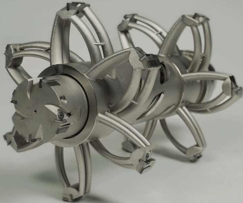
Fig 1: Additive manufacturing brings lightweighting to large-diameter tools, such as this 3D printed tool for machining the stator bore of an electric car motor. A more advanced version of this tool is now in use in the production and manufacturing of electric vehicles.
