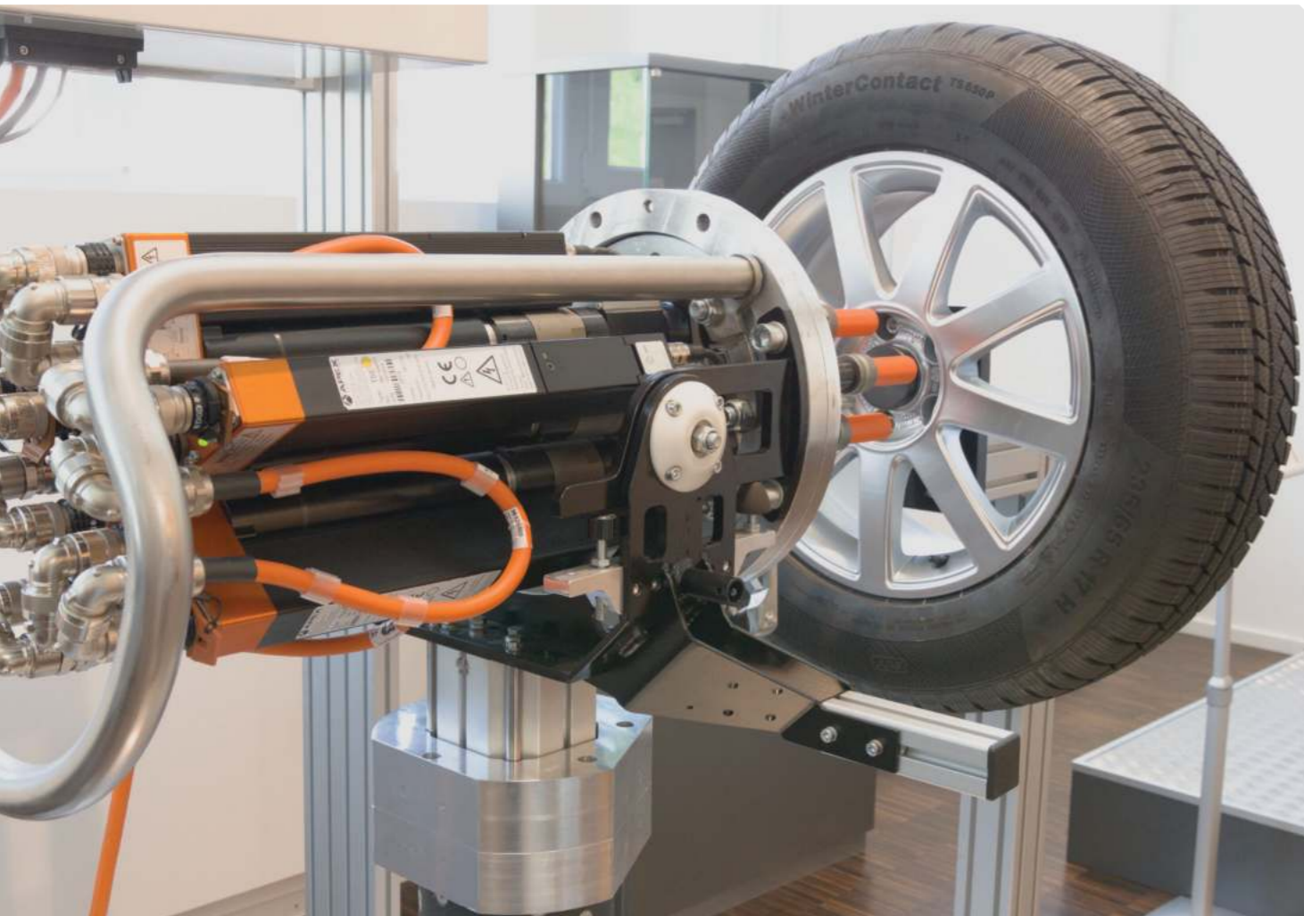
Electrical and pneumatic screw spindles, for example for the automated mounting of vehicle wheels, require the grinding of a large number of different 30 to 650 mm (1.18" to 25.6") long motor and gear shafts with diameters between 3 and 65 mm.
