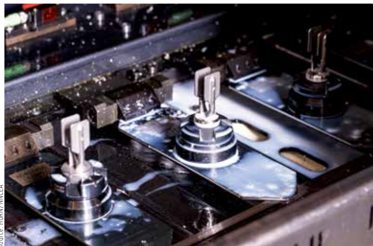
The M fork is used in level indicators.
