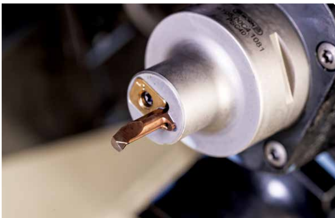
The new Supermini with sintered geometry solved the chip breaking problems.
