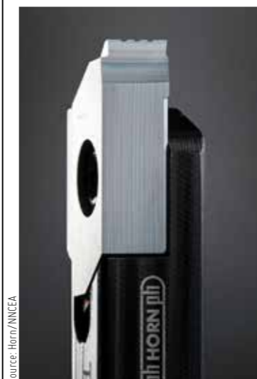
The tool edge is ground to a sharp and precise finish.
