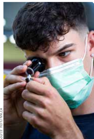
Checking the cutting edges after 22,500 recesses.
