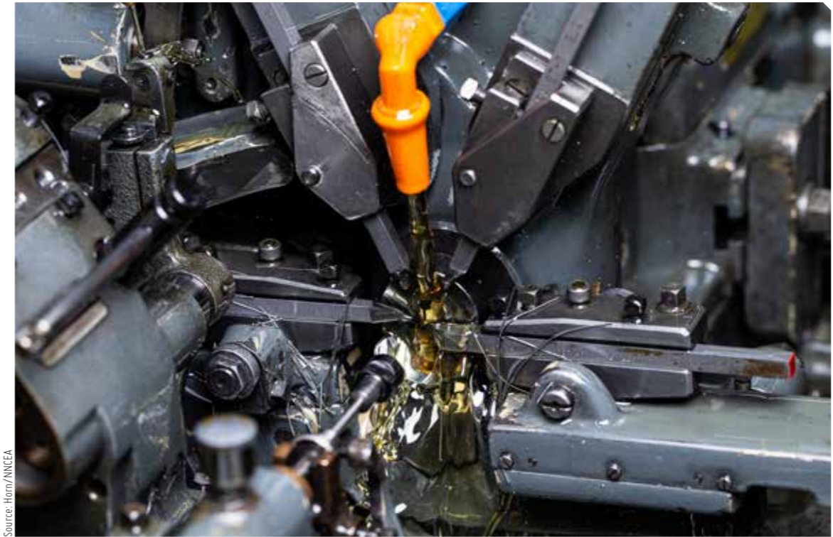
Ticking over like a Swiss watch: Traditional cam-controlled sliding-head lathes are an essential part of large-scale series manufacturing.
