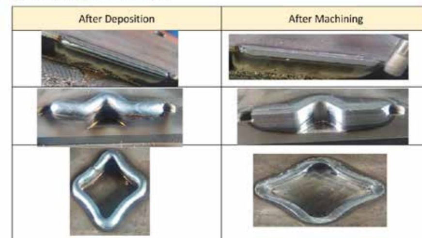
Before/After Images: Photographs showing a component after deposition and after machining to illustrate the transformation from rough WAAM output to precision-finished part. (Reference 'Die-Reclamation' images)
