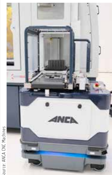
Source: ANCA CNC Machines AIMS Pallet transfer from AutoFetch to the grinder
