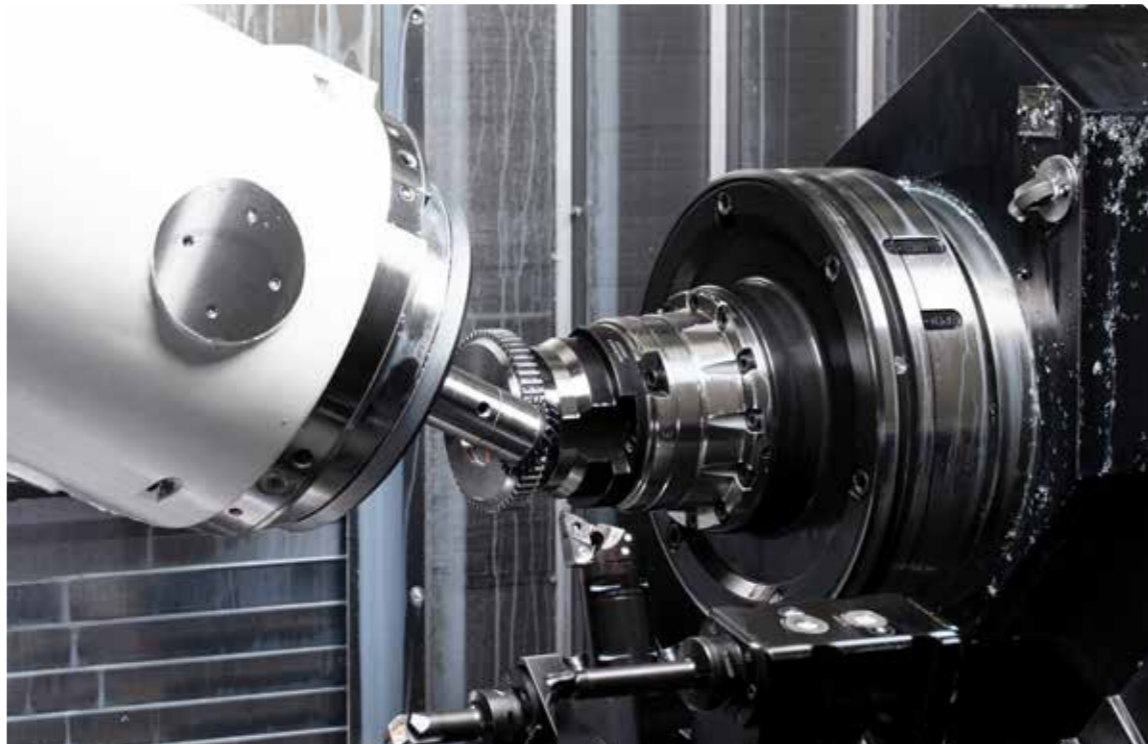
Gear skiving has enabled Collins to make its processes even more reliable while at the same time optimizing the quality of its components.
