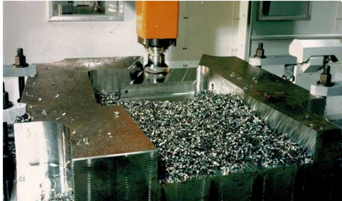
Circa 1999: Dry machining with HSC: High-speed machining entirely without cooling lubricant — what started out as an experiment at the beginning of the 21 st century has become a symbol of resource-saving manufacturing.
