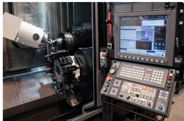
Gear skiving can be easily programmed on modern CNC production centers.
