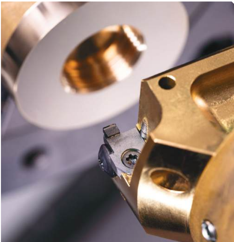
An MCD-equipped S117 system is used to machine the end faces.
