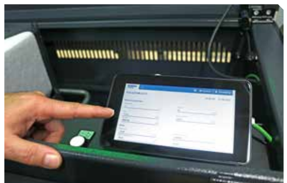
The integrated touchpad enables the monitoring and visualization of the most important operating data for the system.
