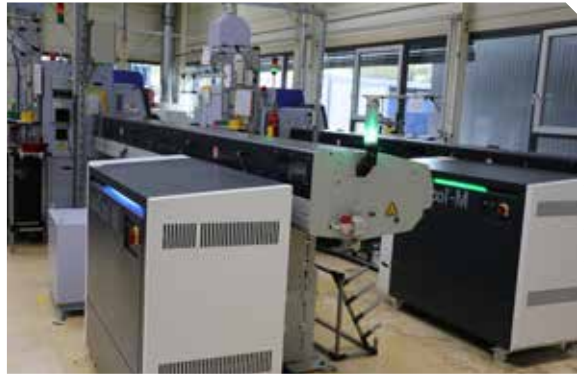
LubiCool®-M units supply the two SP-23 and SV-20R automatic sliding headstock lathes from Star Micronics with cooling lubricant as required.
