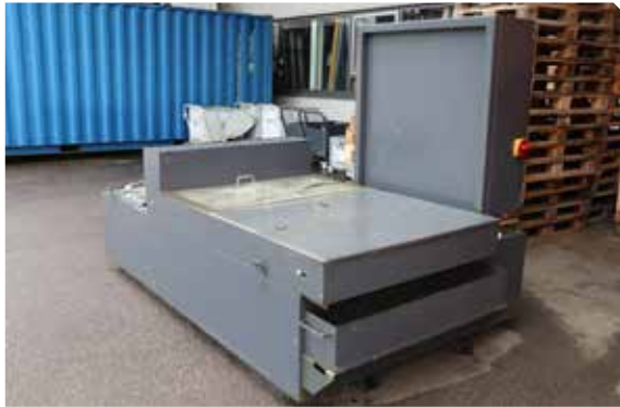
Retired: This high-pressure station with a flat bed filter had to make way for the significantly more compact and powerful KNOLL LubiCool®-L.
