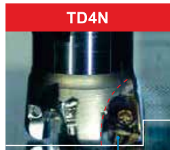
Cutting chips which were discharged well
