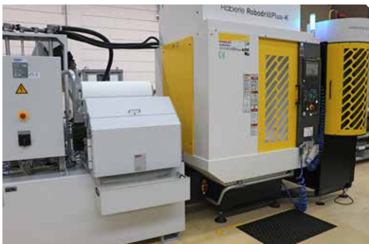
For milling centers that require a larger volume of cooling lubricant, KNOLL offers an open high-pressure system with a greater filter and tank capacity. TROKAMED had the recently delivered automated Häberle Robodril Plus-K equipped with this system.
