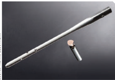
Eccentric turning enables highly productive production of non-round external contours.
