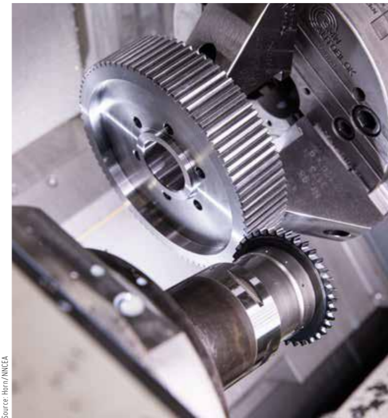
The disc carrier is used in a clutch/brake combination.
