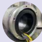
Spindle Motor Winding Encapsulation
