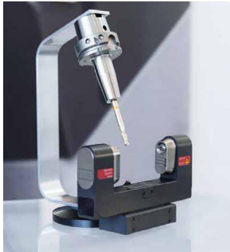
LC50 Digilog — Laser Measurement System from Blum-Novotest
