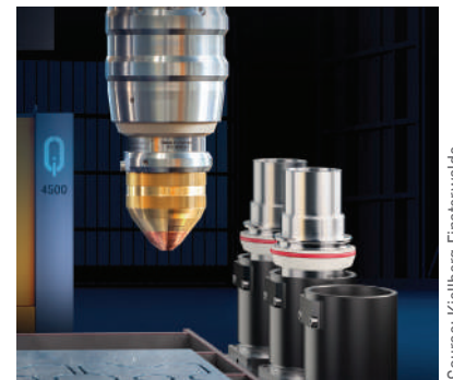
The Q-Torch Auto Change System enables fully automatic changing of plasma torch head.
