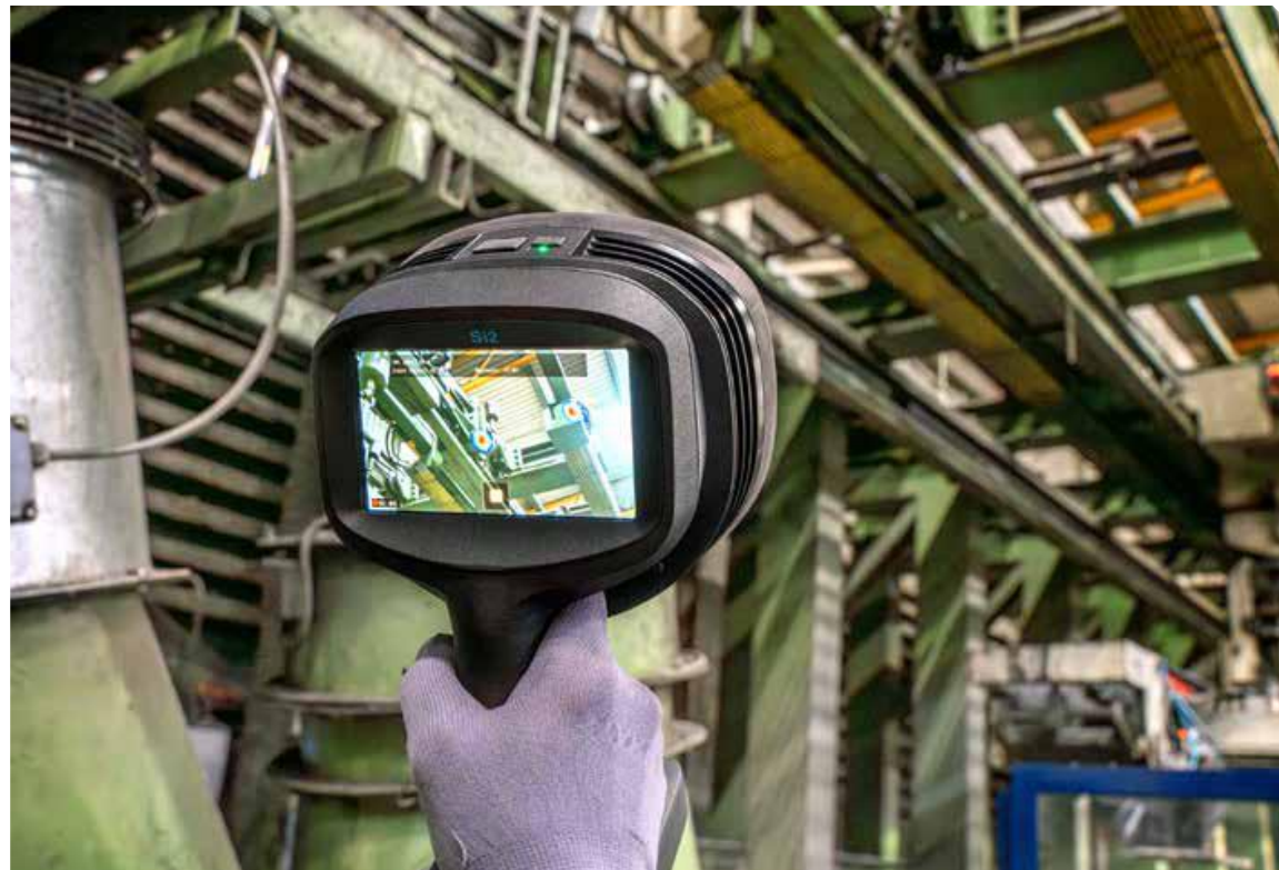
Finding compressed air leaks using acoustic imaging is a fast, efficient way to reduce overall energy costs.
