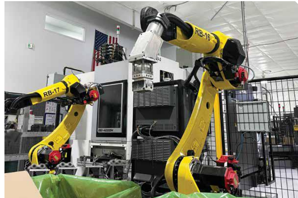
The cell runs unattended during overnight shifts, though not literally 'lights out' due to the vision system's need for light. Tool life management and tool load software from Okuma help prevent crashes and other issues during unattended machining.
