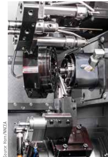
High-speed whirling enables continuous cutting through concurrent turning.
