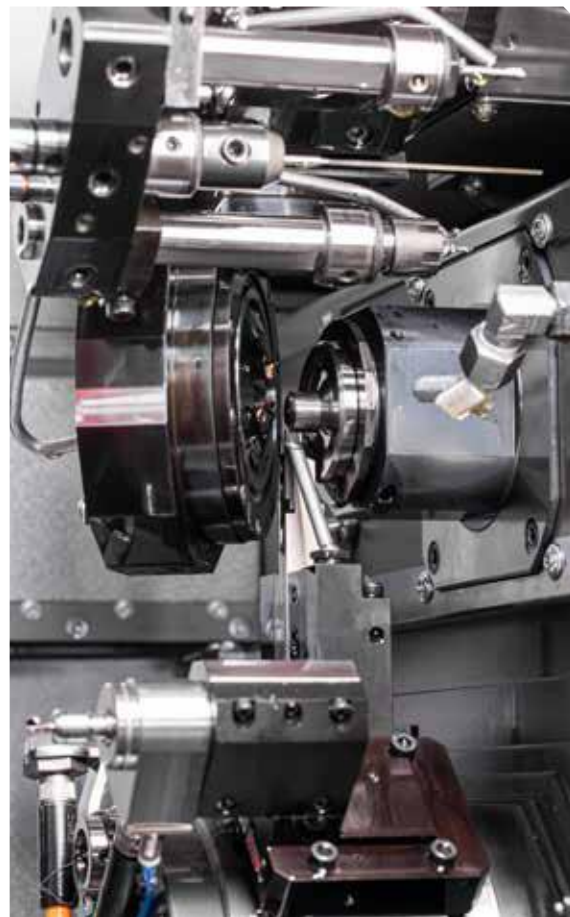
Two whirling heads are equipped for whirling two different threads on a bone screw.
