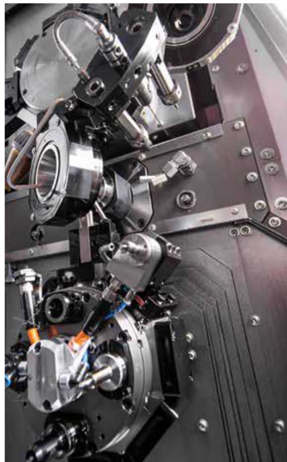
The kinematics of the Swiss-type turning machine allow effective and simultaneous machining with two, three, or four tools.
