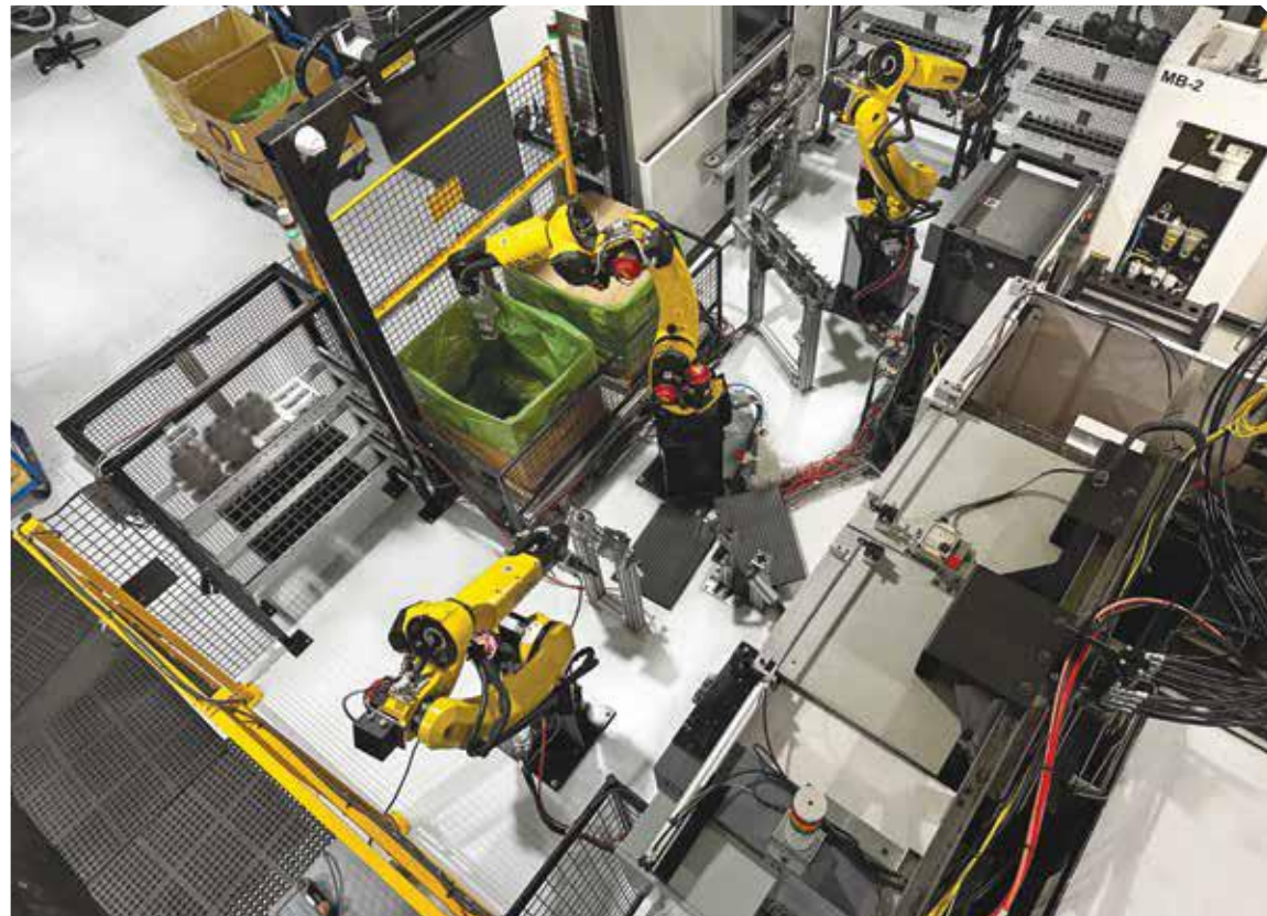
MetalQuest is a precision manufacturer and internal FANUC integrator that recently added its first cell with a 3D vision system. The cell machines castings, which arrive at the cell in boxes from the foundry.
