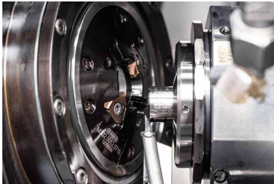
The carbide grade IG35 is used for machining titanium alloys.
