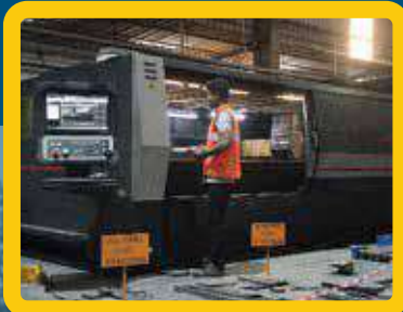
CNC - Amada 9 Kw Fiber Laser
