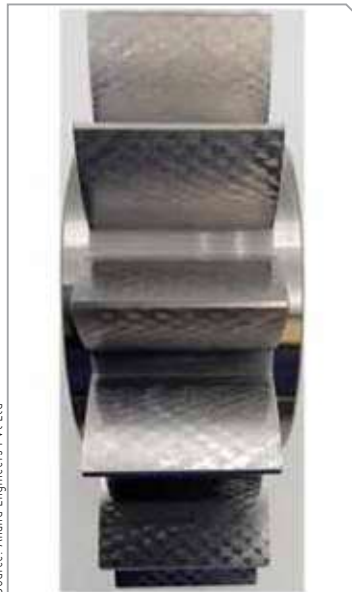
FZG gear picture taken upon completion of 12 load stages
