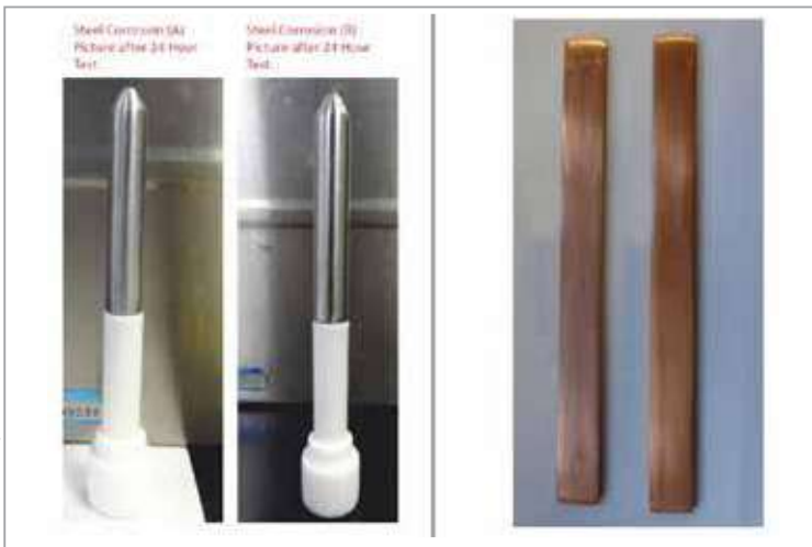
Steel Corrosion Test (ASTM D 665 A and B)
