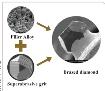
High-vacuum, high-temperature brazing of diamond with a suitable filler
