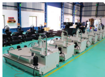
Coolant Tank Assembly Line
