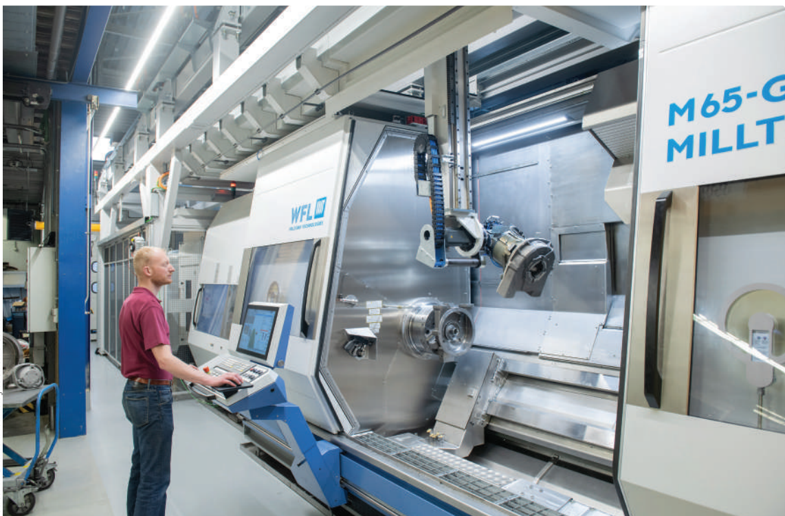
Bredel has fully automated the WFL M65-G Millturn with a gantry loader and a jaw quick-change system. (Photos of Bredel and Tim Wentink)
