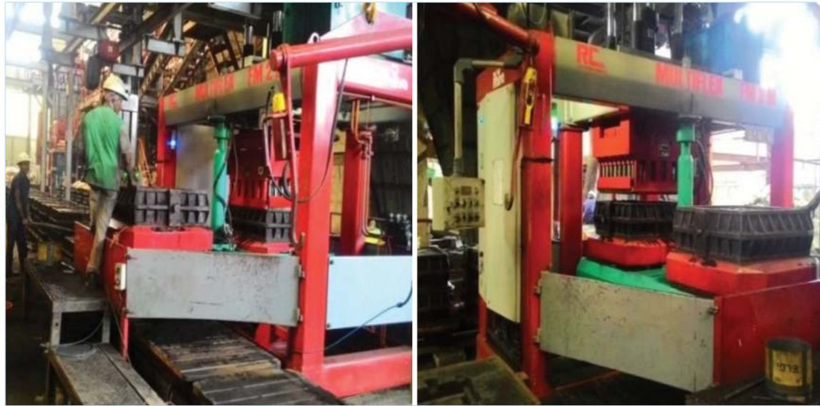
New technology driven production: Reducing use of natural resource – sand by initiating High Pressure Moulding Line – Green sand
