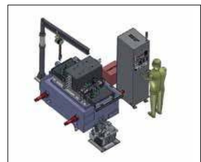
Figure 2: Test Rig for evaluating different flow control strategy
