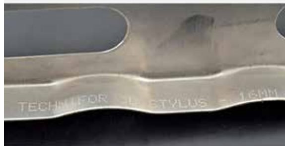
Marking on inclined plane, distorted surface, uneven flatness
