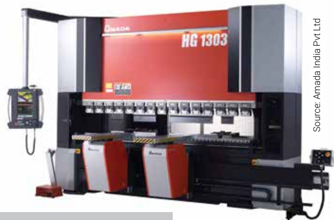
Amada's HG1303 Press Brake with sheet follower.
