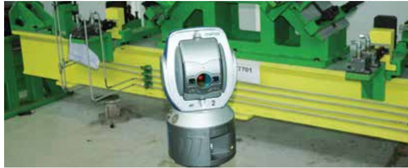
The FARO Laser Tracker Vantage is the ideal laser tracking solution for large volume measurement.
