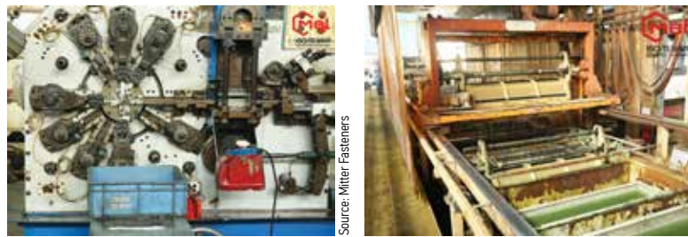
Facilities for Stampings (Multi Slide Part Former)
