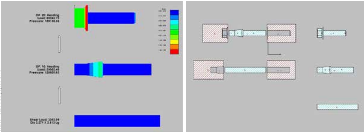
Fig. 5: Hex Progression & Tooling Using NAGFORM
