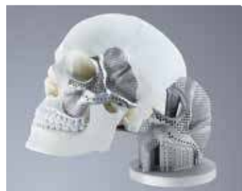
A laser sinters a precisely shaped implant from the powder bed.
