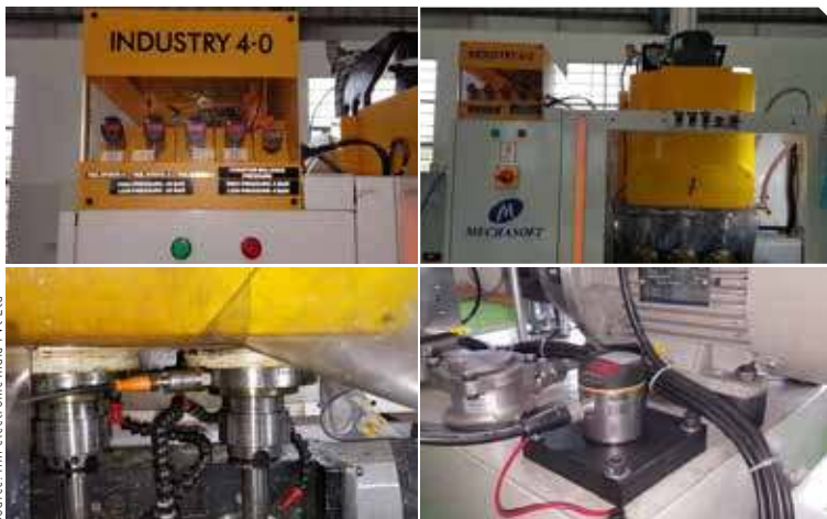
Groove Milling machines with pressure, vibration, level and temperature monitoring in real time
