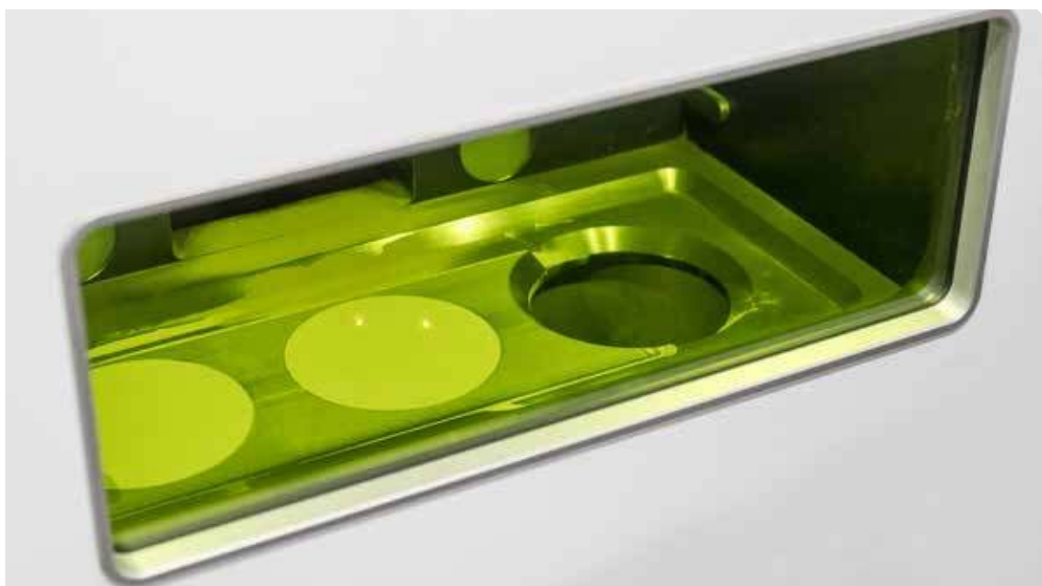
CONMET uses TRUMPF's TruPrint 1000 3D printer to produce customized craniomaxillofacial implants.
