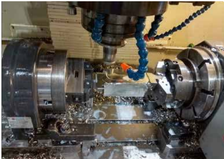
Rough machining on 3-axis machine
