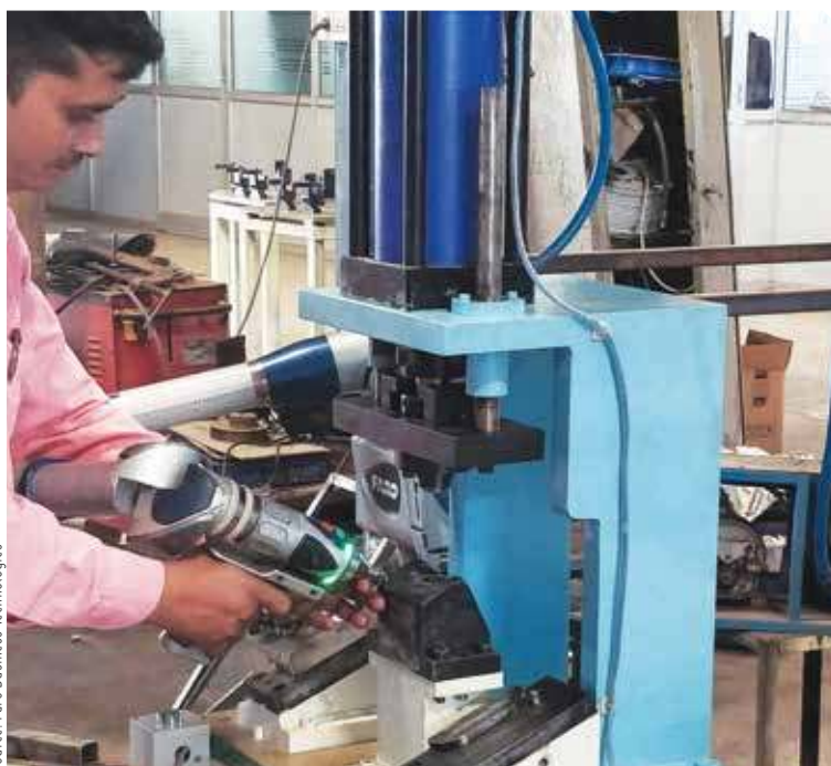
With the FARO Edge, operators no longer have to worry about moving a bulky, heavy object to a measuring room, or about finding a suitable hand tool.
