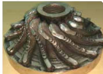
(e) Impeller by conformal slicing
