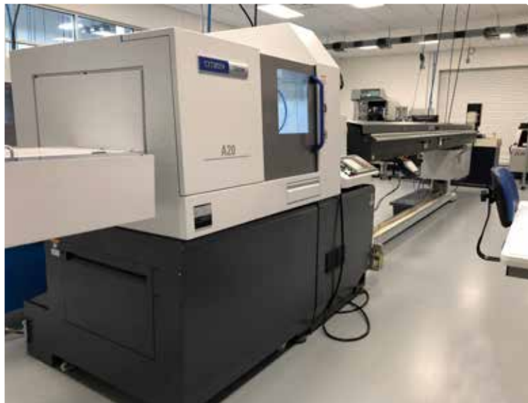
MMD Medical currently uses Swiss-type machines for dry machining of the plastic medical components.
