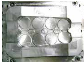
(a) Monolithic injection mold
