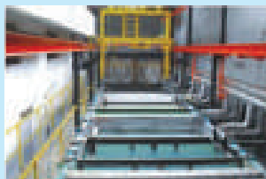
DIP PT PLANT WITH PLC BASED TRANSPORTER
