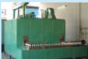
ROTOR CURING OVEN
