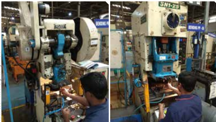
The manual process of feeding single piece in a die mounted on the press
