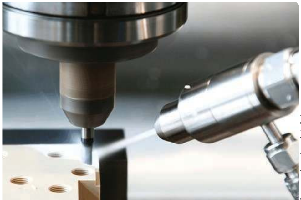
Cooling and cleaning with the quattroClean system when machining PEEK.
