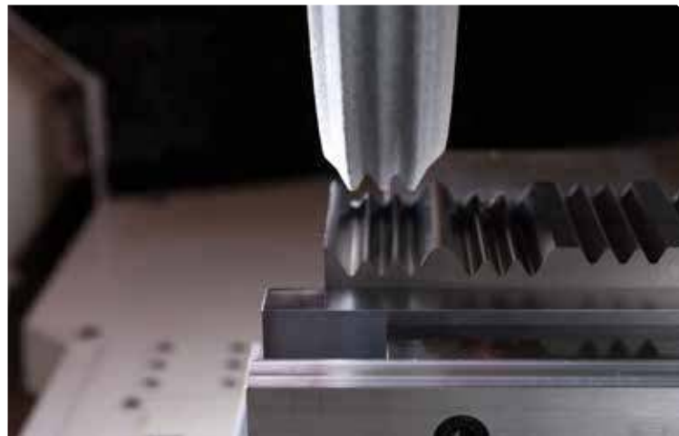
Particularly in hard-to-machine alloys, creep-feed grinding using a profiled wheel offers a way to realize precise forms that would be difficult to generate via any other type of machining.
