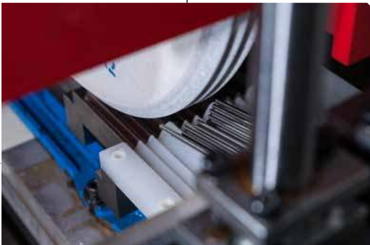
Another consideration for maximizing the effectiveness of coolant in creep-feed grinding: Coolant nozzles arranged to follow the profile of the wheel.
