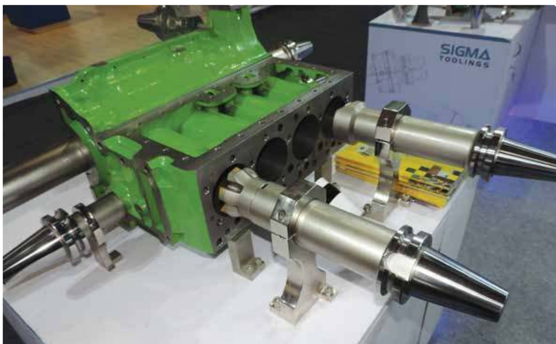
Sigma Toolings' Cylinder block tools demonstrated at IMTEX 2017. (L-R) Crank bore, Cam bore and Linear bore boring bars showing their areas of application
