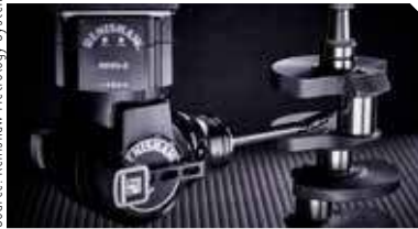
Source: Renishaw Metrology Systems Ltd REVO SFP2 measuring crankshaft
