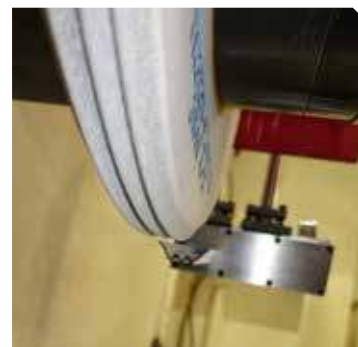
Here is another view more clearly showing the array of coolant nozzles matching the wheel's profile.
