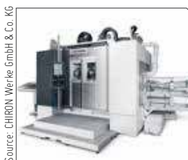
Source: CHIRON Werke GmbH & Co. KG The STAMA 733 series allows all six sides of a workpiece to be machined on a single five-axis center.
