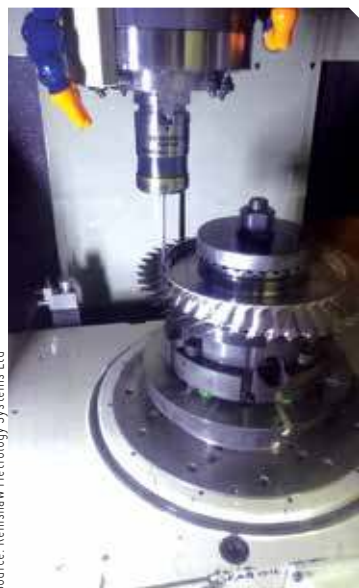
Renishaw's RMP600 high-precision touch probe
