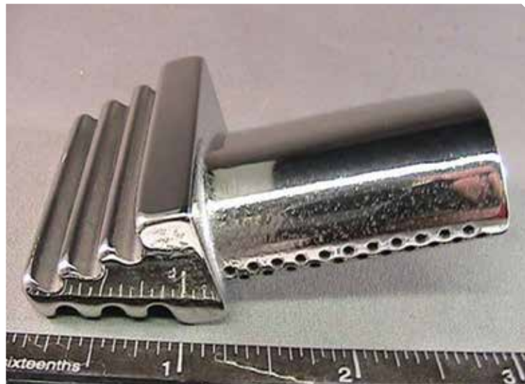
Here, the same blade is pictured following a superpolish postprocessing operation. Imperfections are visible on the leading edge of the profile.
