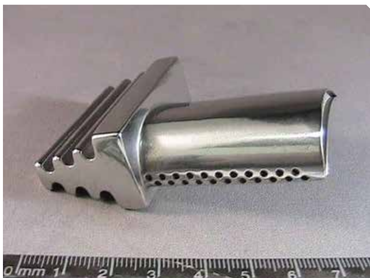
This image shows a second article, built after the feedback loop. The air compressor blade was reoriented to avoid porosity after postprocessing.
