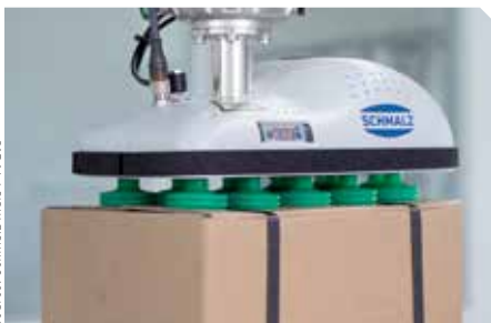
The area gripper FXCB/FMCB is ISO TS 15066-compliant. The gripping surface is available with flexible foam or bellows suction cups; the gripper itself is available with or without integrated vacuum generation.
