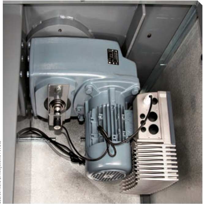
The NORDAC FLEX frequency inverter with its integrated PLC enables safe and highly comfortable bending of rebars to exactly the desired angle.
