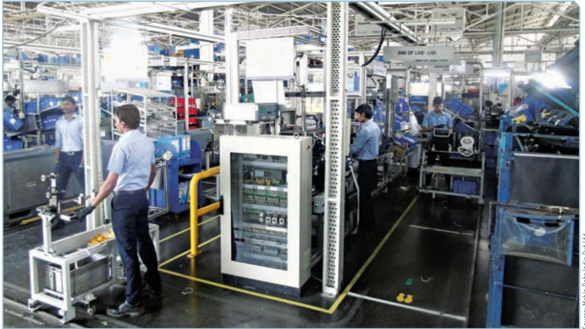
Operator moving along with a fixture trolley starting from the left corner and completing the entire assembly by the time he reaches the right corner.
