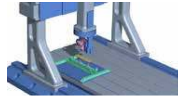
Fig 8. Gantry: Water-jet/mill combination
