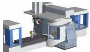
Fig 9. Huron: A good compromise between long reach and rigidity.
