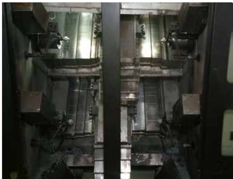
Fig. 1: 4 Spindle Machine → 2 spindles (left) for Operation and 2 spindles (right) for Loading Unloading
