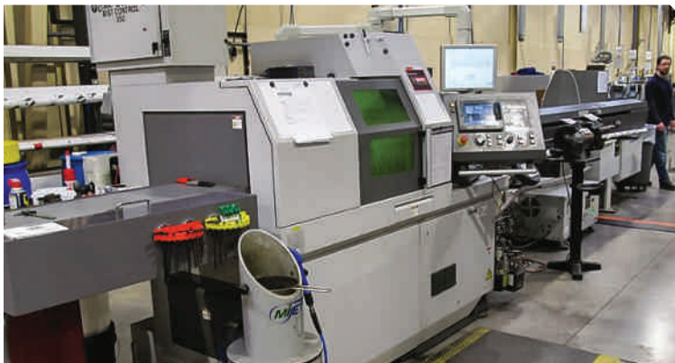
Paragon Medical — Southington's first laser Swiss machine, a Citizen L220 Type 8, was installed in 2016. Development of laser cutting processes continues to open new avenues of business for the shop.
