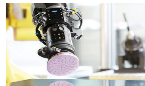
REMENDO automates deburring, polishing and grinding processes
