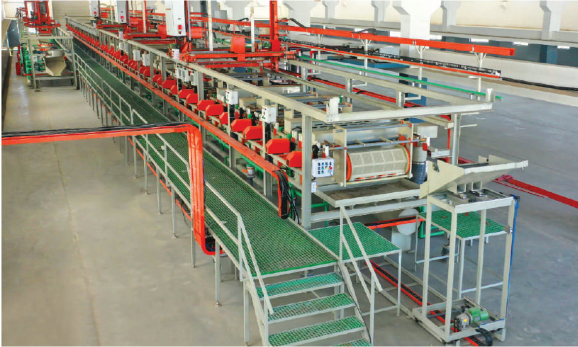
Surface Treatment - CQI 11 Qualified along with REACH and RoSH Zinc Electro Plating Plant
